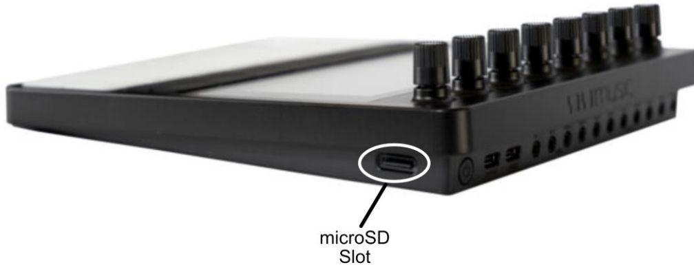
Figure 1-2: microSD card slot location
