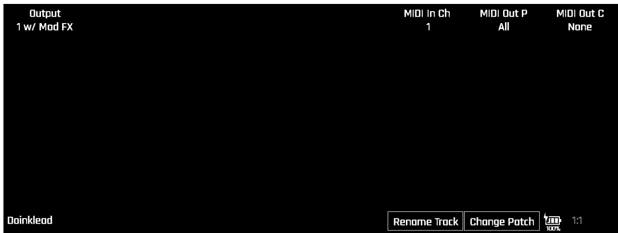
Figure 6-5: Track Configuration screen showing MIDI In Ch parameter setting
