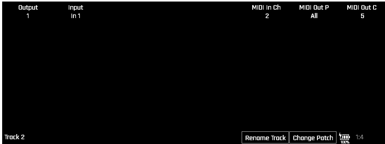
Figure 13-4: MIDI Out Ch parameter in External Track Config Screen
