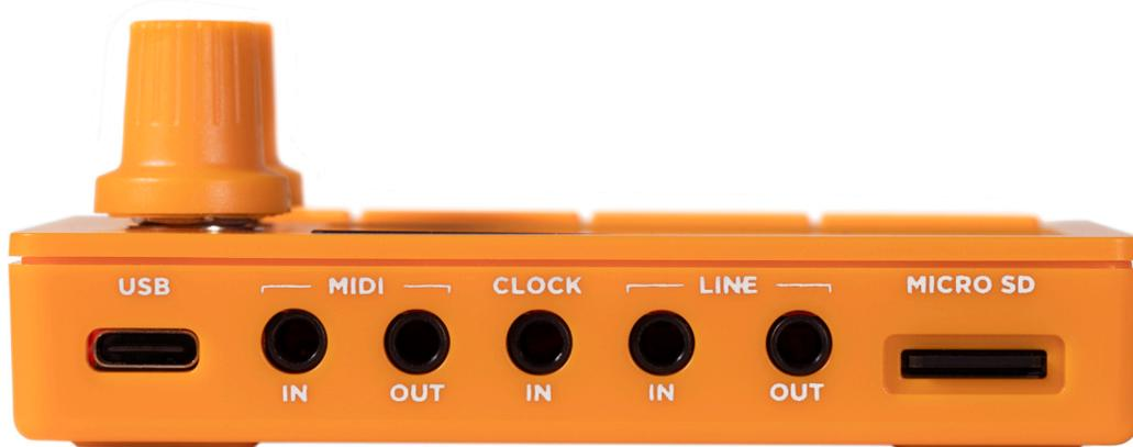
The tangerine MIDI In can be connected to devices that support TRS MIDI Type A or Type B. You can also use the included TRS MIDI Adapter to connect to MIDI 5 Pin DIN controllers.
