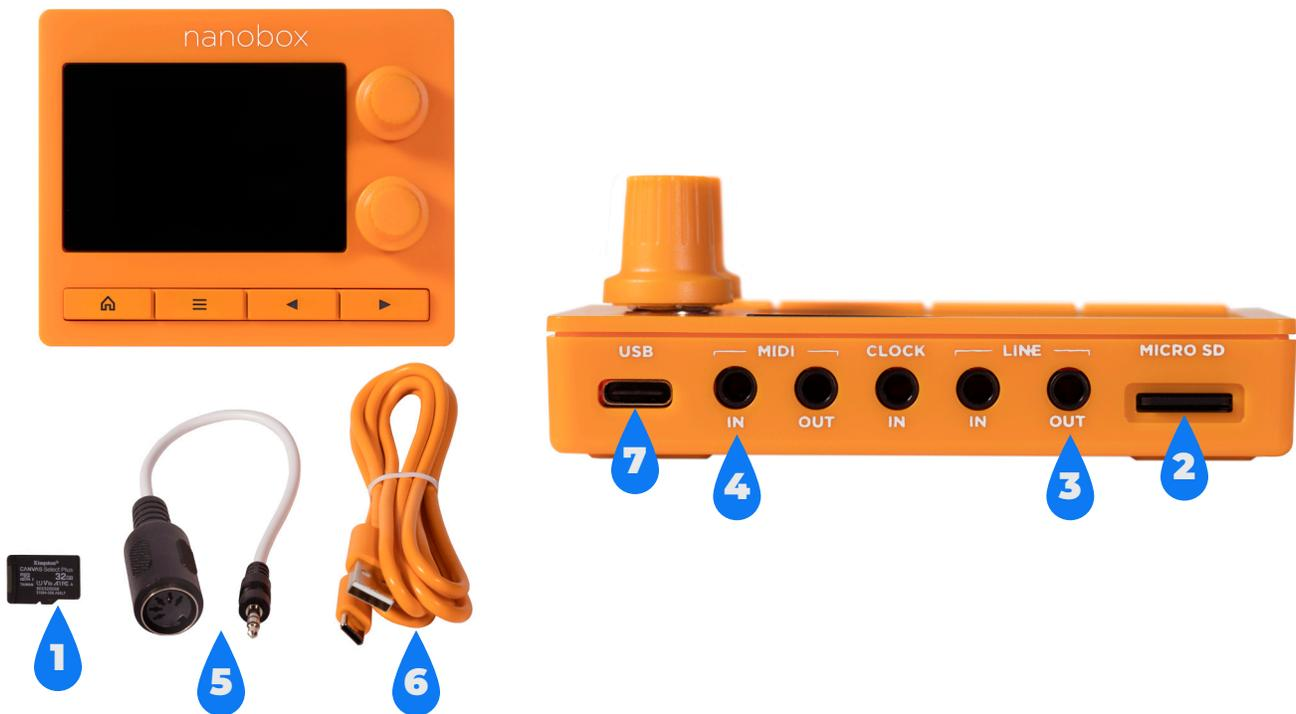
4. Connect the USB power cable (6) to the USB port (7). The tangerine can be powered by a standard 5V, 500 mA USB power adapter or USB battery. The tangerine will start up as soon as it receives power. There is no power button.
