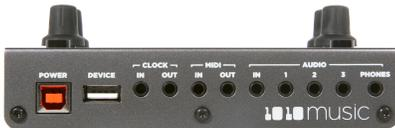
To get started with blackbox, insert the microSD card in the front slot, plug it in, and connect it to speakers or headphones. The microSD card slot is along the short front panel. The power jack and audio outputs are on the back panel. To start, we recommend connecting external speakers or headphones to the PHONES jack, since all outputs are routed to the PHONES jack. Blackbox streams WAV files from and saves your work on the microSD card.
